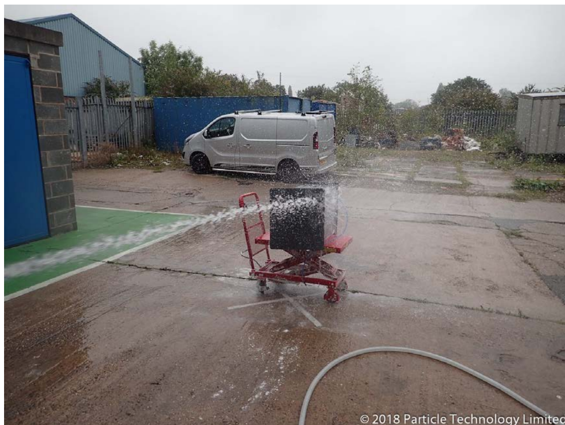
Figure 12 – EUT undergoing IPX6 testing
