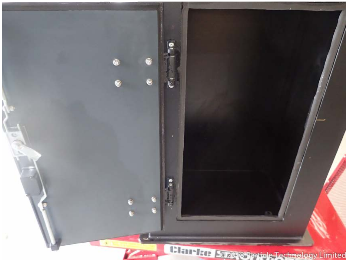
Figure 17 – Inspection showed no visible water ingress on completion of IPX6 testing
