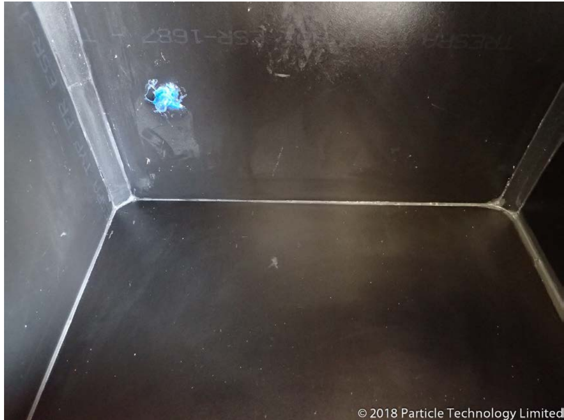
Figure 9 – Enclosure showed no visible dust ingress
