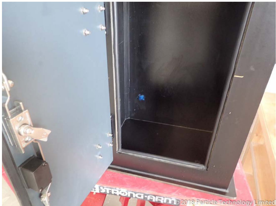
Figure 7 – Enclosure showed no visible dust ingress
