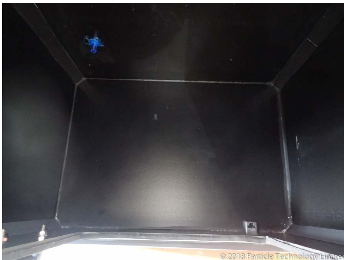
Figure 19 – Inspection showed no visible water ingress on completion of IPX6 testing
