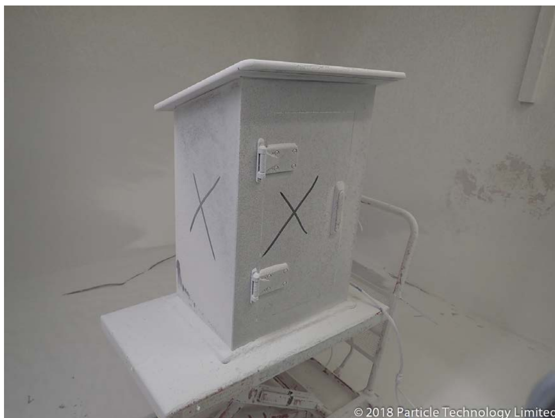
Figure 5 – EUT on completion of IP6X testing
