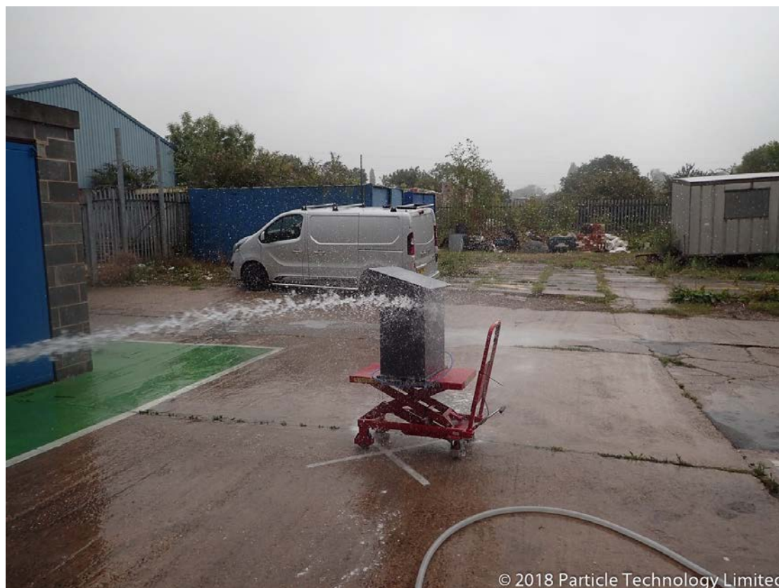
Figure 13 – EUT undergoing IPX6 testing
