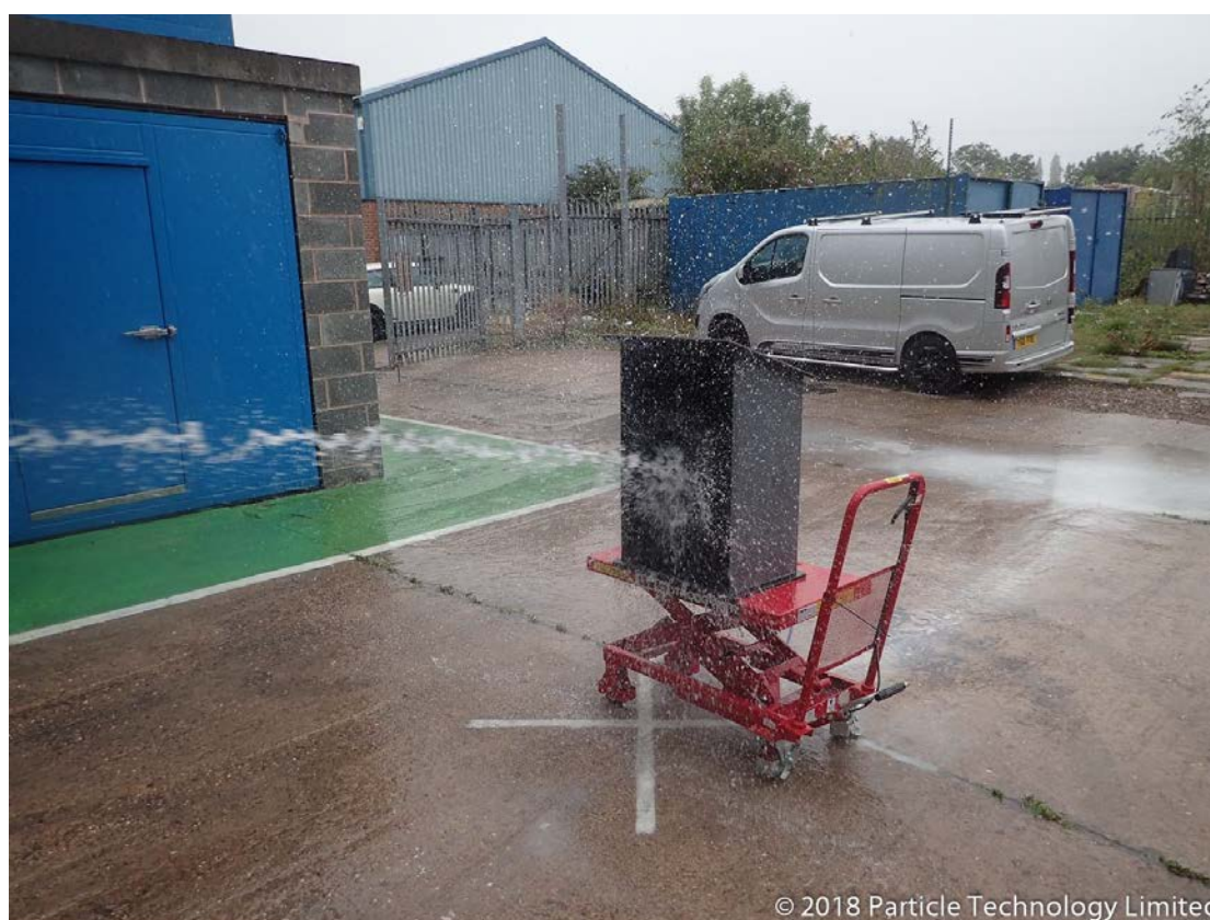
Figure 16 – EUT undergoing IPX6 testing
