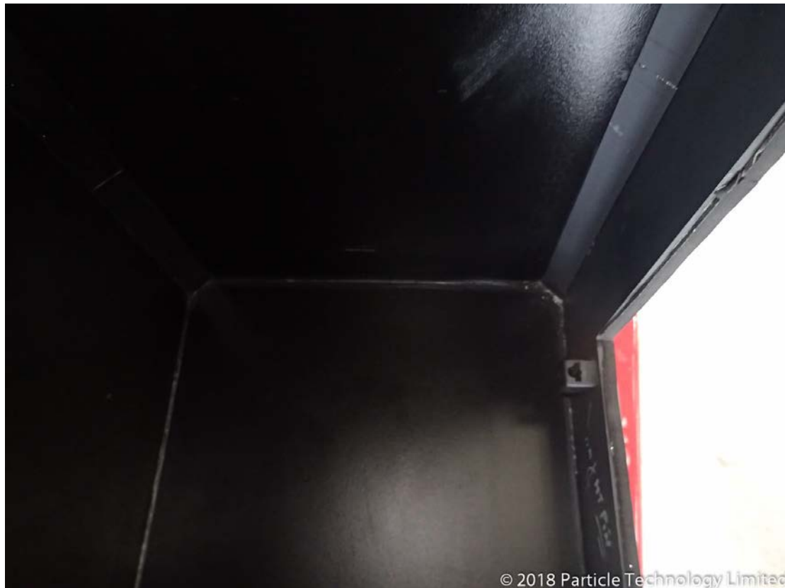
Figure 18 – Inspection showed no visible water ingress on completion of IPX6 testing
