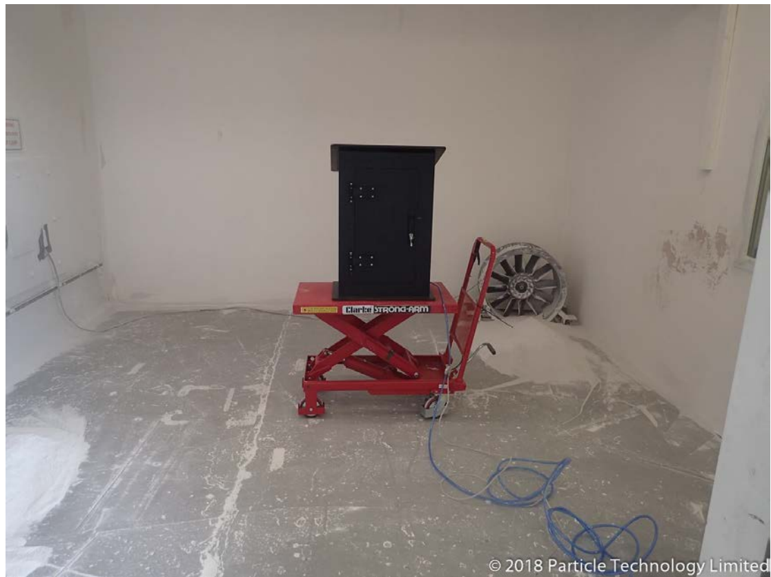
Figure 2 – EUT at the start of IP6X testing
