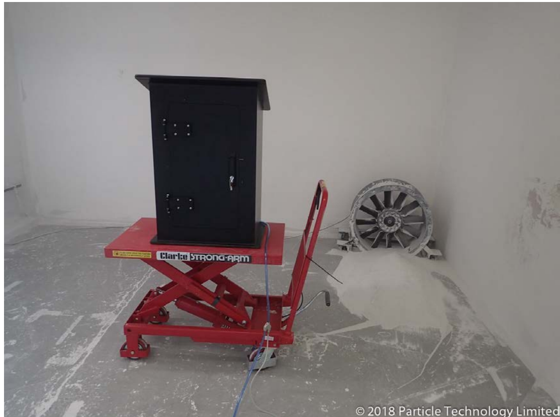
Figure 1 – Arrangement of EUT in IP6X Test Chamber
