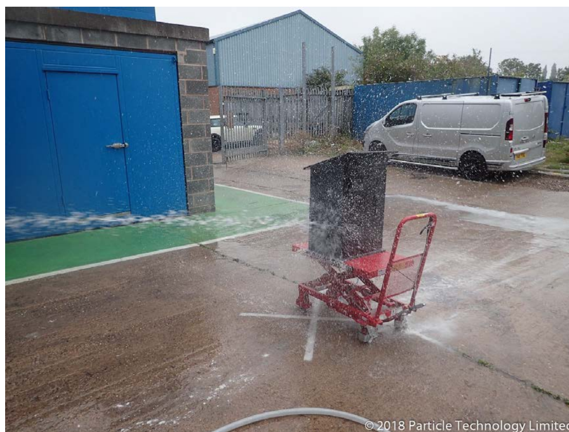
Figure 14 – EUT undergoing IPX6 testing
