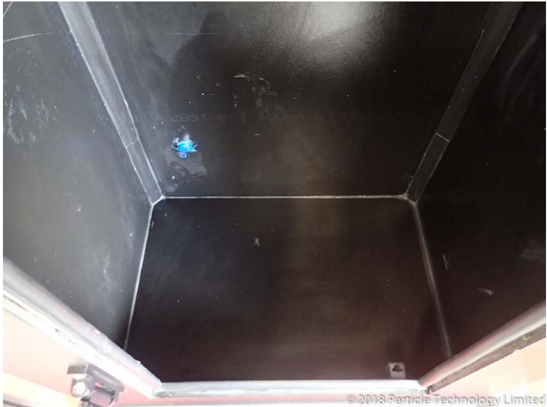
Figure 8 – Enclosure showed no visible dust ingress
