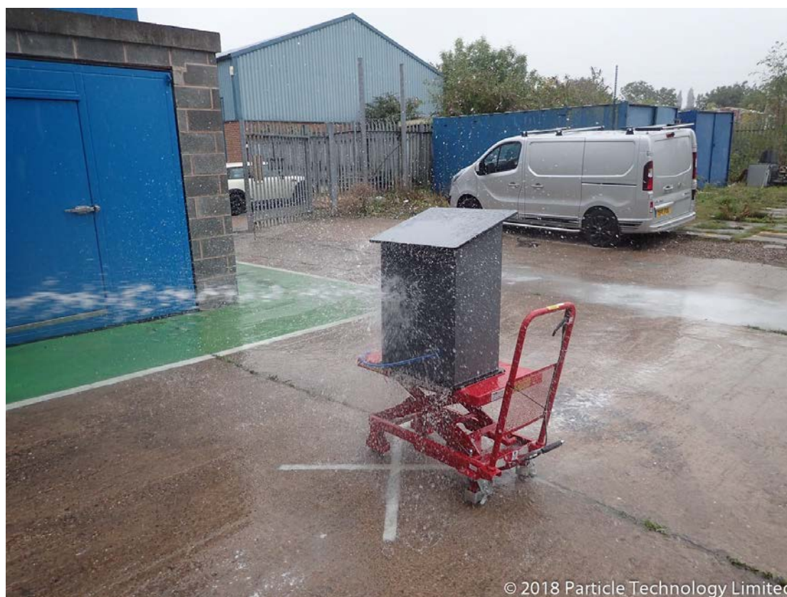
Figure 15 – EUT undergoing IPX6 testing
