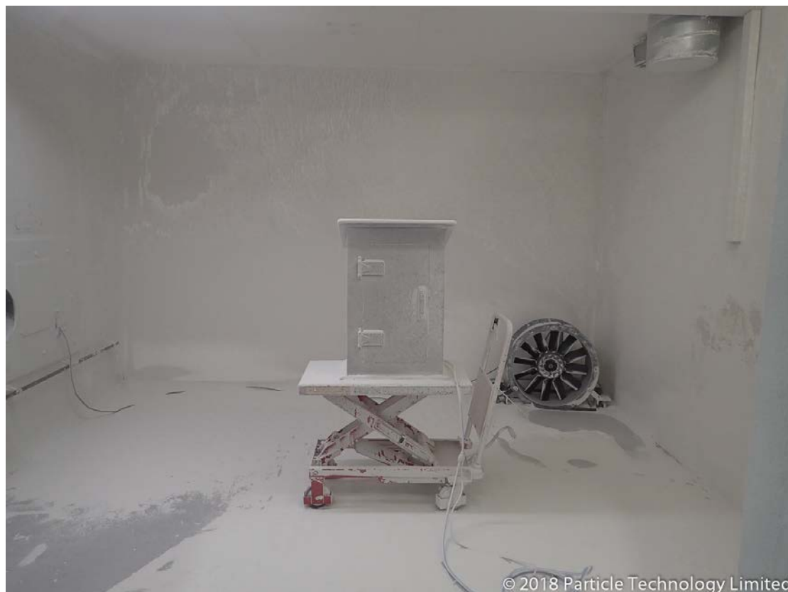
Figure 4 – EUT on completion of IP6X testing
