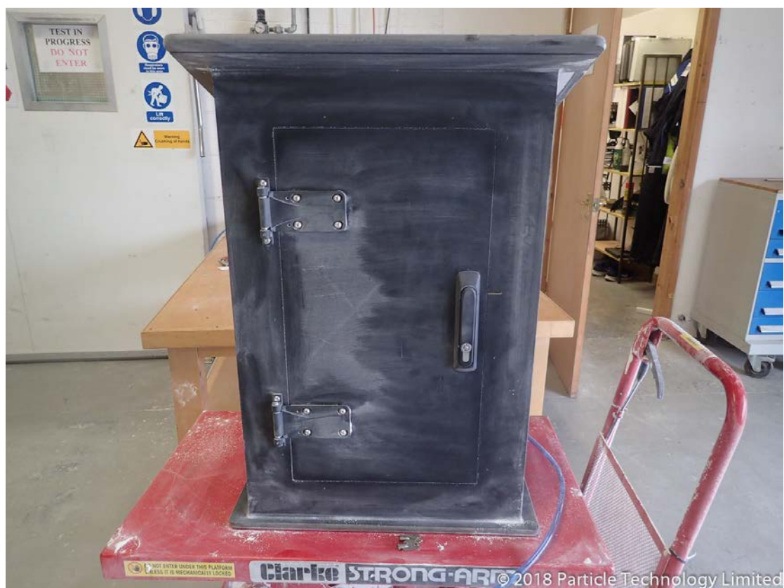
Figure 6 – EUT on completion of IP6X testing
