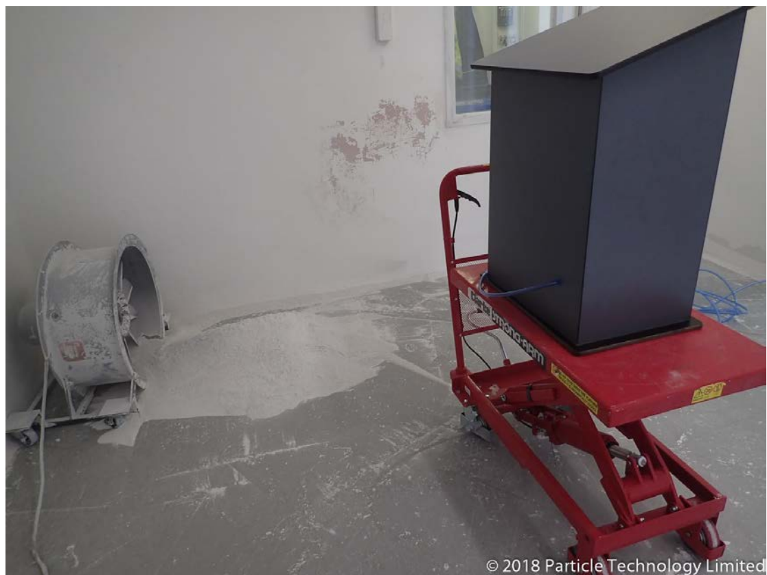
Figure 3 – EUT at the start of IP6X
